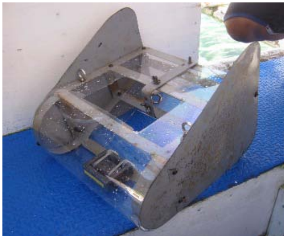
Figure 1: "Teardrop" is a boat-towable, finned hull for holding a video camera. It is lowered beside a boat by a rope and towed to capture videos of coral reefs along a coast.
