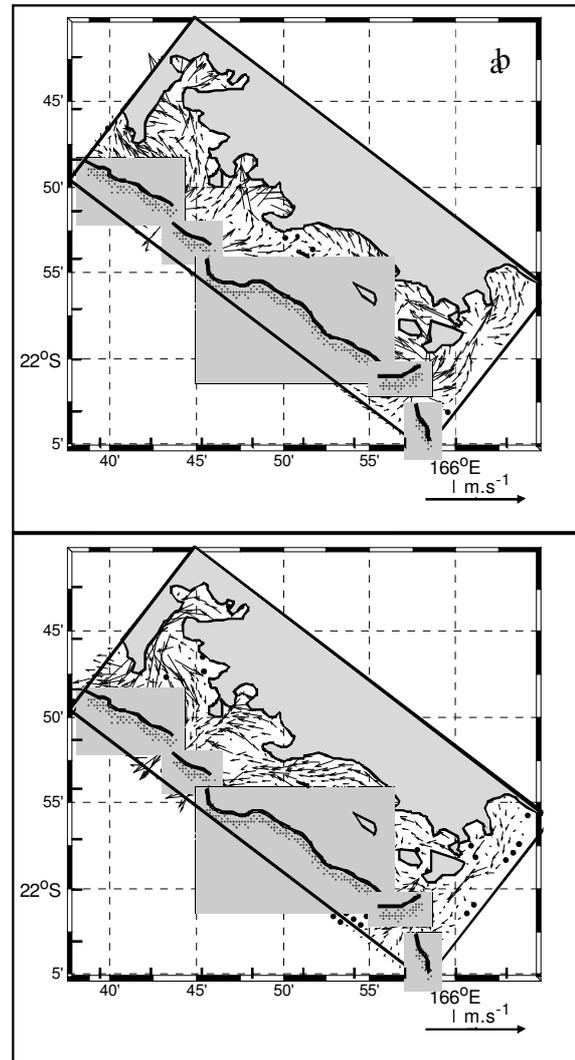
Figure 4: Circulation in the Ouano lagoon, on the 2012, July 16<sup>th</sup>, if a cross-reef in-flow is imposed: during the flood (a) and the ebb (b).
