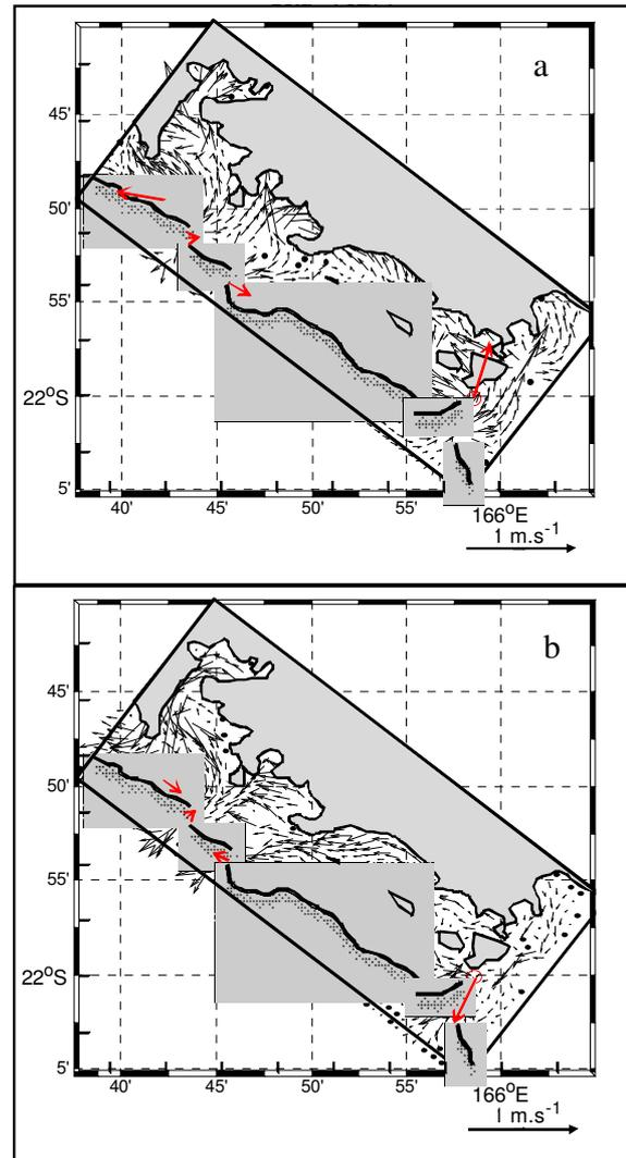
Figure 2: Circulation in the Ouano lagoon during the flow (a) and the ebb (b), on the 2012, July 16<sup>th</sup>. Reference model: the reef has been considered as an impervious wall. Red quivers correspond to measured velocities.
