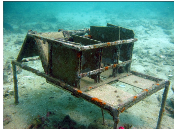
A. An iron frame with settlement panels
