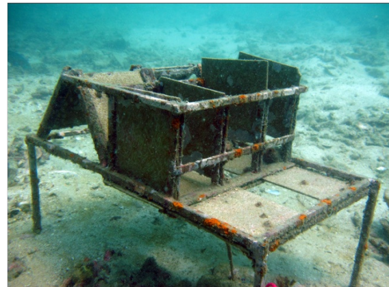
A. An iron frame with settlement panels
