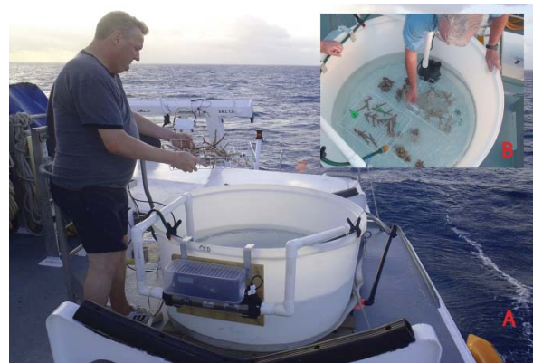
Figure 1: Experimental set up on the top deck of RV Cape Ferguson. A) Side view showing the relative size of the tank and the in-line temperature control unit. B) Top view (insert) of the tank showing the arrangement of coral fragments placed at the bottom.
